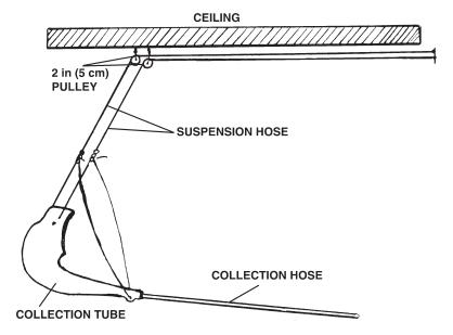
The above diagram illustrates one of the methods used in hanging the rubber suspension harness. The use of pulleys makes it more flexible.
